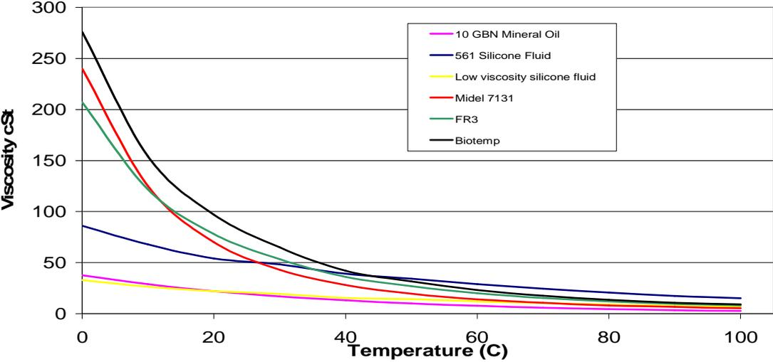
Figure 3.6 – Comparative viscosities with varying temperature
