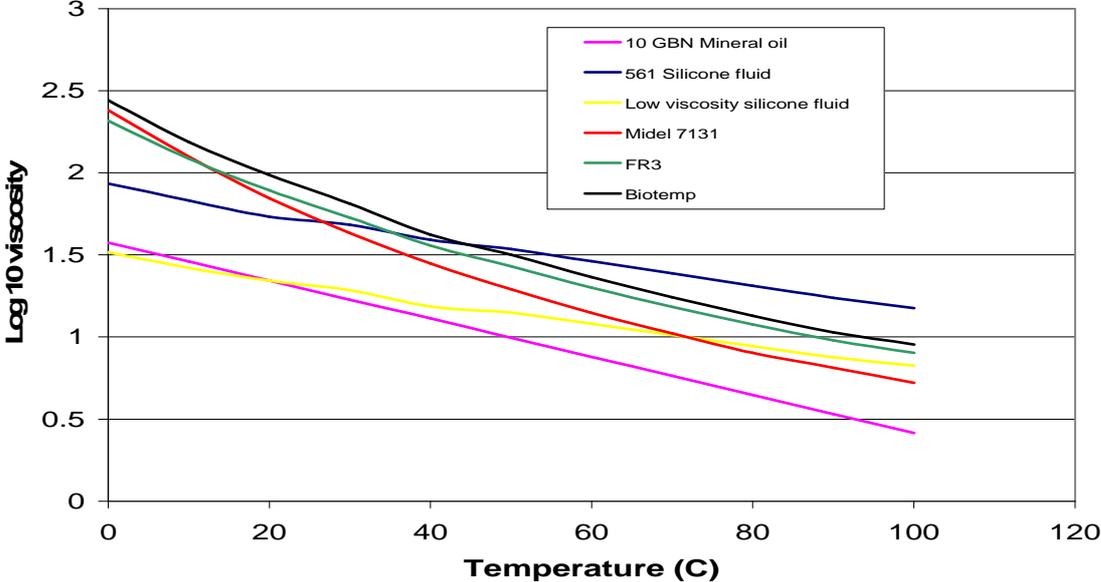
Figure 3.5 – Log<sub>10</sub> (viscosity) vs temperature
