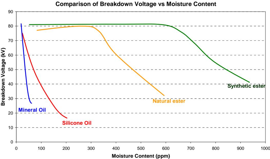
**Figure 4.1 – Effect of absolute moisture content on AC breakdown strength of clean fluids**
