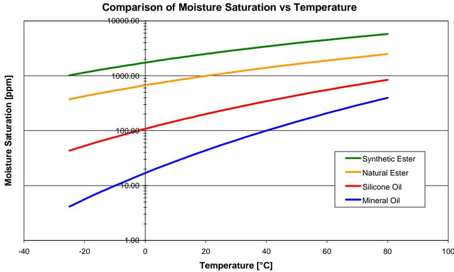
**Figure 3.8 – How moisture saturation varies with temperature**
