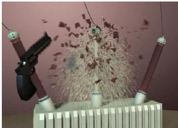
a) Porcelain can explode under internal arcing
