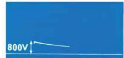
With Metrosil (type 300A/S1) passing 10mA connected across the coil
