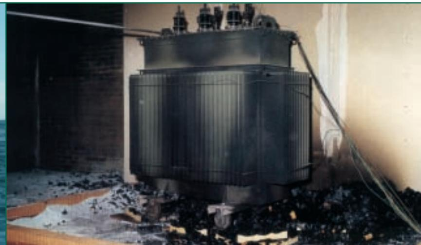
Figure 4. Without contributing to the fire incident, this ester-filled transformer has stood in a veritable bonfire for 70 minutes in the laboratory of the German insurer Allianz. (Courtesy: M&I Materials)
