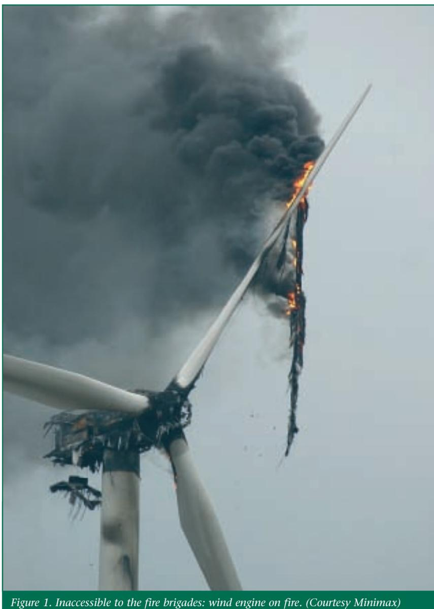
Figure 1. Inaccessible to the fire brigades: wind engine on fire. (Courtesy Minimax)
