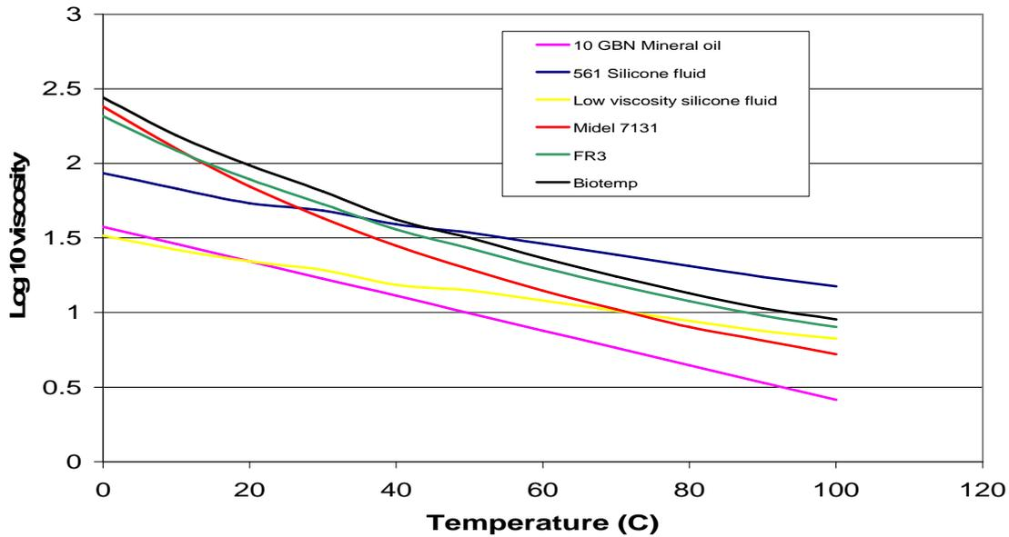
Figure 3.5 – Log<sub>10</sub> (viscosity) vs temperature
