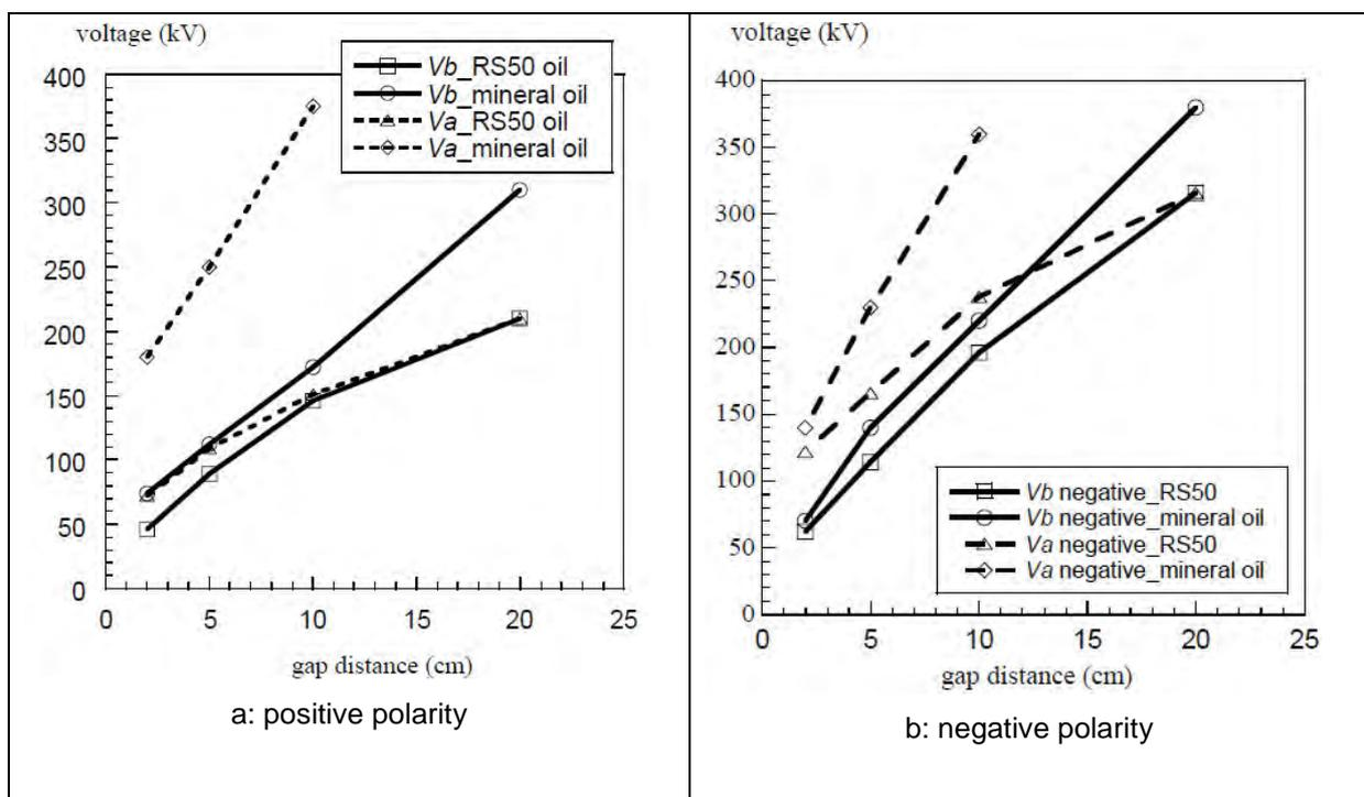
**Figure 4.8: Breakdown voltage ( $V_b$ , 50% probability) and acceleration voltages ( $V_a$ ) for positive (a) and negative (b) voltages for mineral oil and a specific rape-seed based liquid. (Point-to-plane gap, fast rise time/long tail impulse)<sup>65</sup>**
